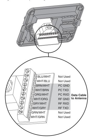
Figure 18: Switchplate Wiring - Antenna Power Cable
